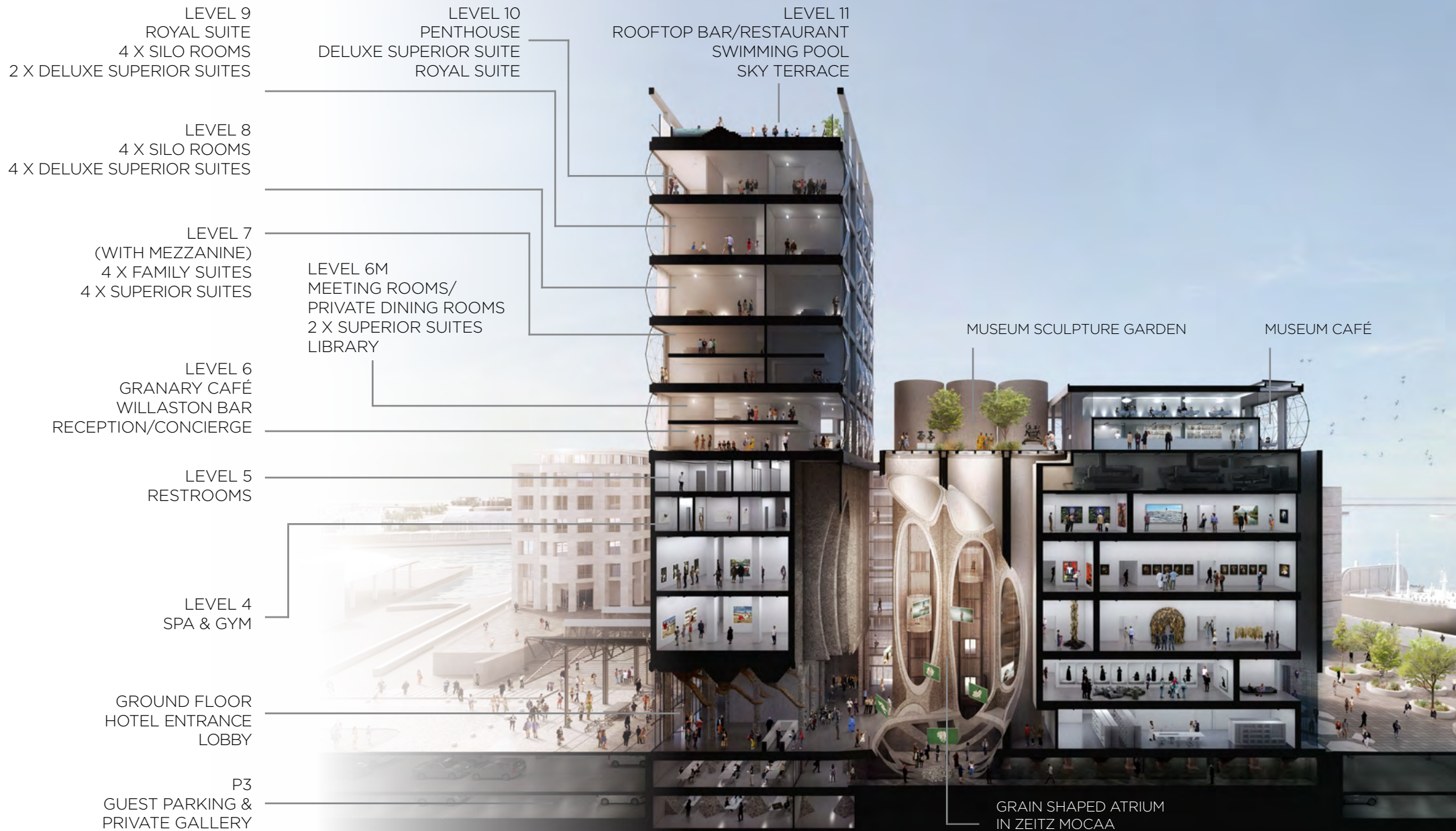
A cross-section of the entire grain silo building, which is comprised of Zeitz MOCCA and The Silo Hotel
